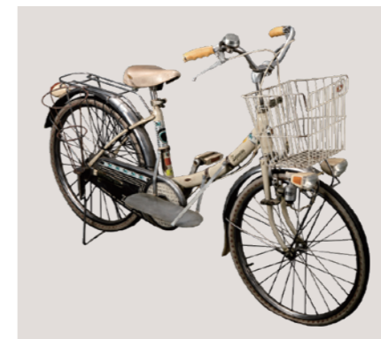
A single-pedal bicycle This bicycle that has been modified so that it can be pedaled with only one leg since a prosthetic leg does not move.
